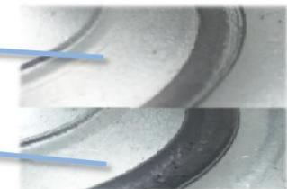
Non-quenched Ball Track's abrasion and gap clearly.
